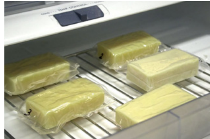
Milk Casein Plastic: Biodegradable. Edible. 500x better at keeping oxygen away from food. 12
