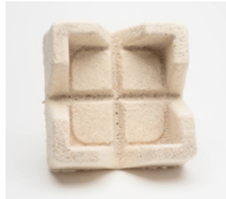
Mushroom® Packaging: Made from mycelium and the agricultural byproduct of hemp. It's a high-performance packaging solution that's cost-competitive with conventional foams, yet 100% home compostable. 11
